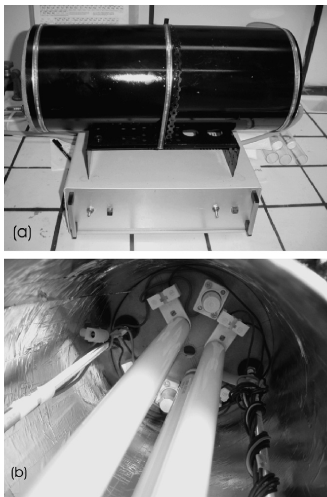
Fig. 1. The photocatalytic packed bed reactor (PPBR) used in this study: (a) outer and (b) inner views. Operation is possible with four or two lamps.
